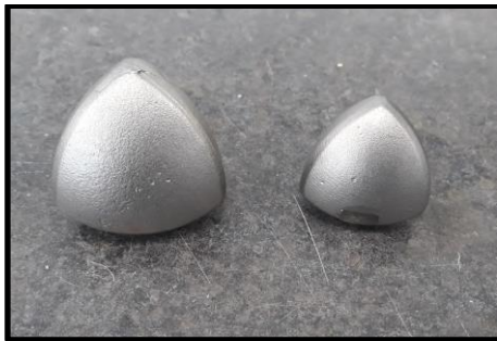
Figure 7- Photo of steel RGM
