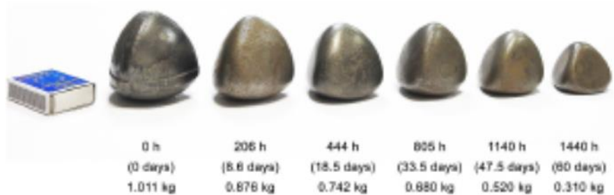
Figure 4 - Photos of RGM charge samples taken during the Rudozem test
