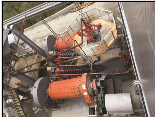
Figure 3 - Photo of the two tumbling mills at Rudozem lead-zinc concentrator, Bulgaria
