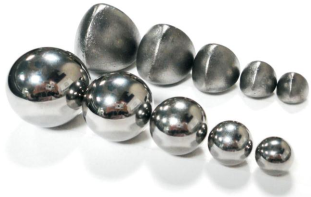
Fig. 2: A comparison of two types of grinding bodies in the size of 5 - spherical and model Relo body-C1, used in the tests of the Bond Mill.
